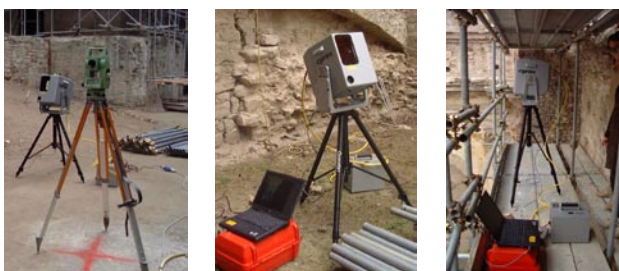
Figure 4. Laser scanner setup
